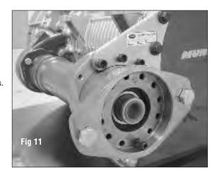
**12.** Remove the cap plug from the end of the PTO output shaft and make sure splines are greased. PTOs are supplied with appropriate grease from factory. If dry apply an anti-fretting compound to splines. Installation of the extended shaft is complete. **Fig 12**
