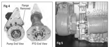
Remove the hydraulic flange (pump end view) from the extended shaft for ease of installation. Set the flange and capscrews aside for re-use. **Fig 4**
