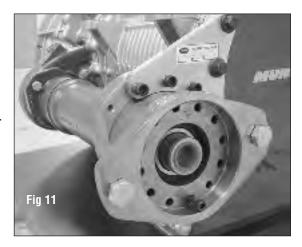
Property of the extended of the PTO output shaft and make sure splines are greased. PTOs are supplied with appropriate grease from factory. If dry apply an anti-fretting compound to splines. Installation of the extended shaft is complete.
